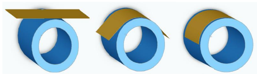
Figure 1. An illustration of the mirror forming process. Time and temperature progress from left to right. The whole process takes place inside an electric oven meeting stringent temperature uniformity requirements.
